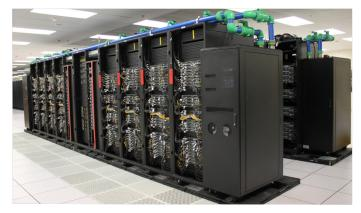
Magma, with 760 compute and user nodes plus 12 management and file access nodes, is a liquid cooled supercomputer built by Penguin Computing featuring Intel® Xeon® Platinum processors and Intel® Omni- Path Architecture fabric. (Photo courtesy Lawrence Livermore National Laboratory/Meg Epperly)
