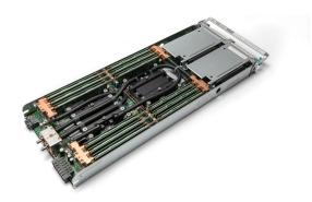
Innovative cooling technology offers high serviceability and provides very stable liquid cooling across the DIMMs.
